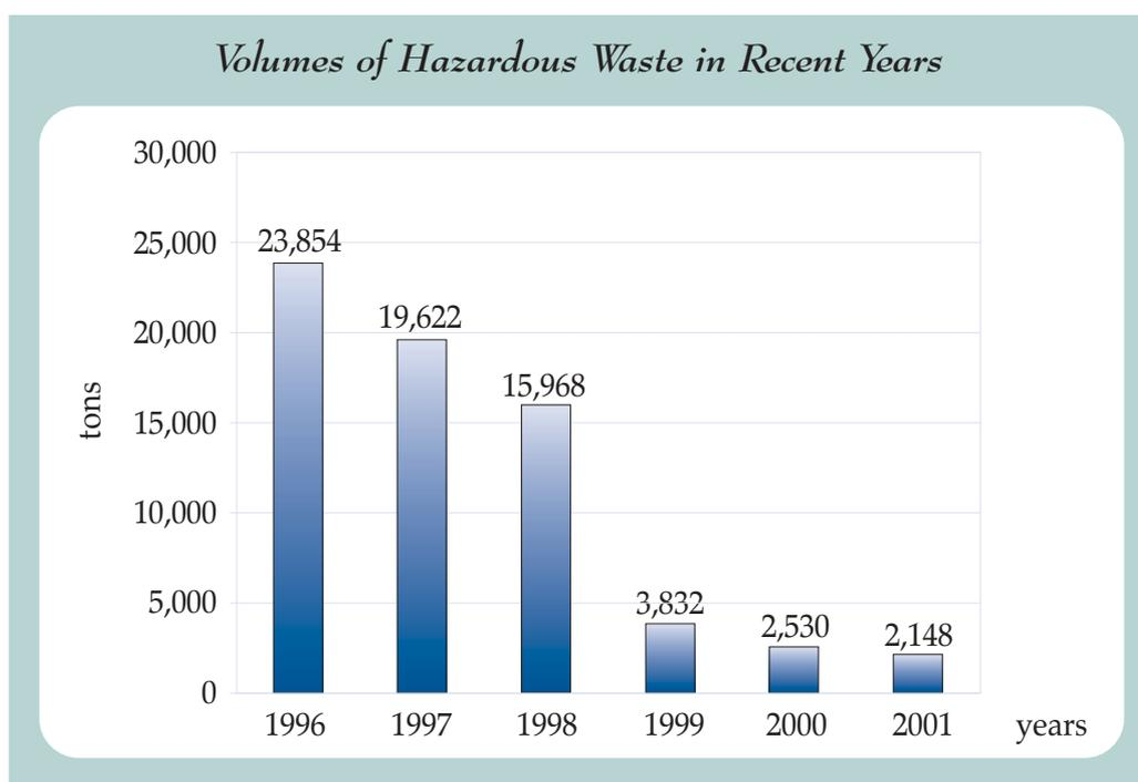
The substantial reduction after 1998 essentially resulted from a new technique to remove water from the sludge during sewage treatment.
