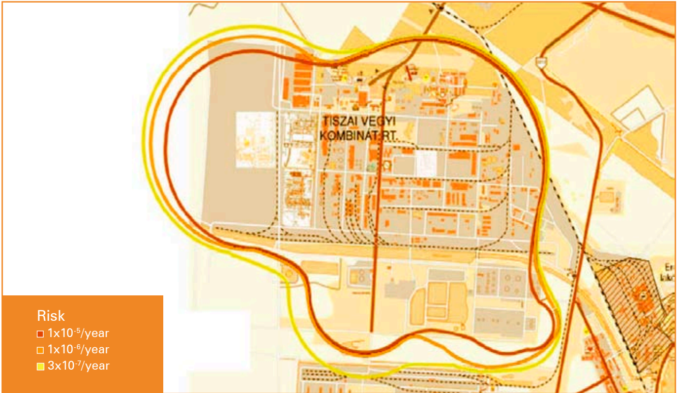
Risk curve envelopes of peak events (Apparently, threats hardly penetrate beyond the TVK fence)
